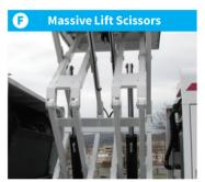
Massive double "X" style lift scissors & 4-corner hopper lift ensure exceptional hopper stability when dumping wet, unbalanced, or sticky debris.
