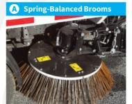
Spring-balanced, free-floating main & gutter brooms automatically apply correct surface pressure for maximum broom wear life. In-cab gutter broom electric tilt is standard.
