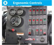
Vertically-mounted control panel is 6-way adjustable for easy & ergonomic viewing. One-touch sweeping allows for operator to preset functions. Brooms raise automatically in reverse.
