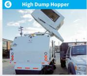
Variable dump height hopper (up to 12' high) with 44" extra-long dump door easily reaches most dump trucks.
