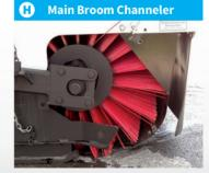
Main broom channeler (optional) effectively sweeps large quantities or bulky & light debris (leaves/pine straw). Self-adjusting as main broom wears.
