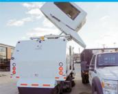
Variable dump height hopper (up to 11' high) with 44" extra-long dump door easily reaches most dump trucks.
