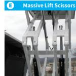
Massive double "X" style lift scissors & 4-corner hopper lift ensure exceptional hopper stability when dumping wet, unbalanced, or sticky debris.
